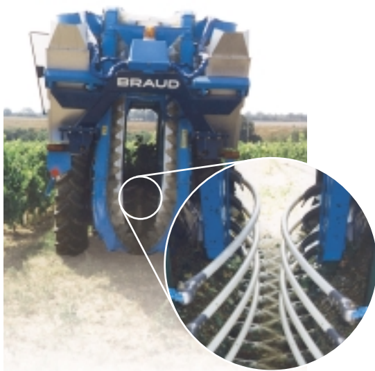
ERTALON 66 SA “shaking rods” on wine-grape harvester.
